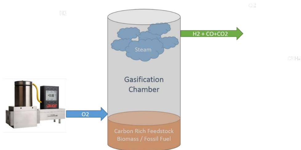
Syngas is typically created from three major components: carbon, oxygen and steam. The carbon and steam are created by heating the fuel, and the oxygen is artificially introduced.
