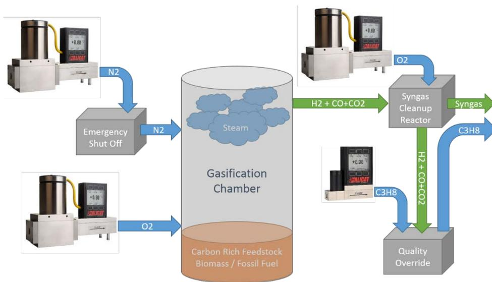
When working at such high temperatures with potentially combustible materials, purging the system quickly is sometimes necessary for safety. A safety shut off system can easily be configured with a mass flow controller to flood the chamber with nitrogen. These controllers can be built with a CSA Class 1, Division 2 (ATEX zone 2) area classification to ensure that local fire safety regulations are being met.
