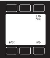
Press **TARES** to access **TARE FLOW**. Press BACK to return to the Tares display. Push MAIN to return to the Main display.
