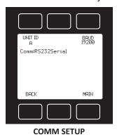
**UNIT ID** – Valid unit identifiers are the letters A-Z and @. The identifier allows you to assign a unique address to each device so that multiple units can be connected to a single RS-232 or RS-485 computer port.
