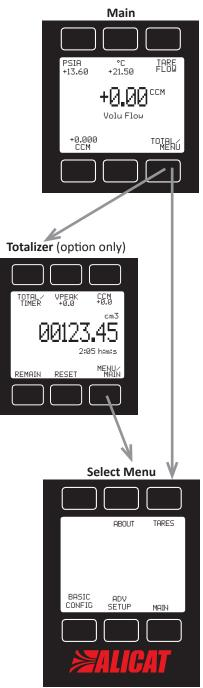
The **Main** display shows pressure, temperature, and volumetric flow. Pressing the button adjacent to a parameter will make that parameter the primary display unit.
