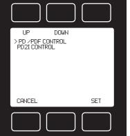
PID Values determine the performance and operation of your proportional control valve. These terms dictate control speed, control stability, overshoot and oscillation. All units leave the factory with a generic tuning designed to handle most applications. If you encounter issues with valve stability, oscillation or speed, fine tuning these parameters may resolve the problem.
