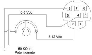
Controllers: A simple method for providing setpoint to controllers
