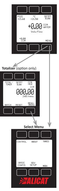
The **Main** display shows, temperature and volume flow. Line pressure will be also be displayed if the meter was order with this option.
