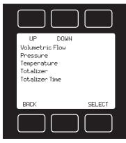
Press **DEVICE UNITS** to access menus of units of measure for each parameter (and totalizer if so equipped). Scroll to the desired unit and press select. Once selected, you will see the message shown below. Verify that all connected devices expect the change. See pages 40 and 41 for a full list of available units.
