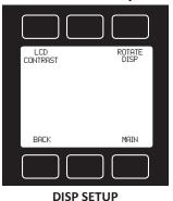
**LCD CONTRAST:** The display contrast can be adjusted between 0 and 28, with zero being the lightest and 31 being the darkest. Use the UP and DOWN buttons to adjust the contrast. Press SET when you are satisfied. Press BACK to return to DISP SETUP.
