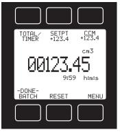
TIMER button will cycle the large numbers on the display between total volume and time elapsed.
