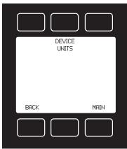
Press **BASIC CONFIG** to select device units Press **BACK** to return to the Select Menu display. Push **MAIN** to return to the Main display.
