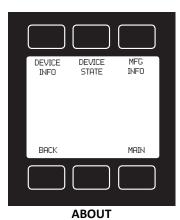
Press **DEVICE INFO** to show important information about your flow device including the model number, serial number, and date of manufacture.
