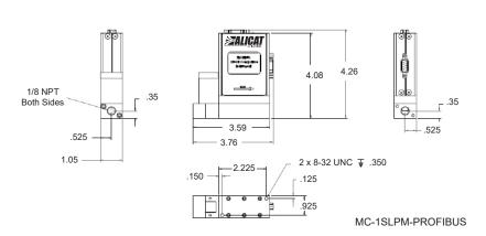
PROFIBUS MC1SLPM shown to provide PROFIBUS connector dimensions only. Flow body and valve dimensions will vary with range. Please see Alicat's device specifications for complete dimensions.
