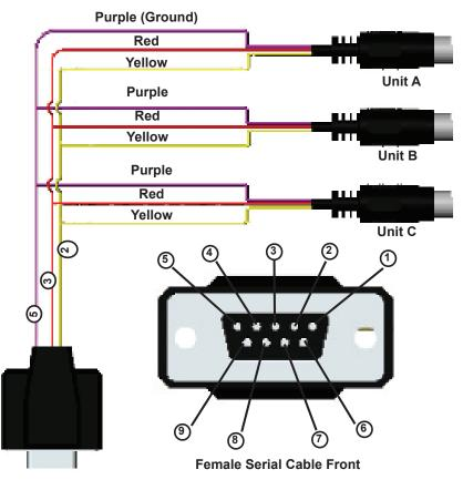
Typical Multiple Device (Addressable) Wiring Configuration
