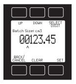
To activate Batch Mode: Press BATCH. Then use SELECT DIGIT to move the arrow to the desired digit, and the UP and DOWN buttons to change the value. Press CLEAR to return to zero. Press SET to record your value. If the controller has a non-zero Setpoint, flow will start immediately. If not, press SETPT to select a Setpoint.
