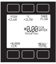
The following parameters are displayed in the **Main** mode: Pressure; Temperature; and Volumetric Flow.
