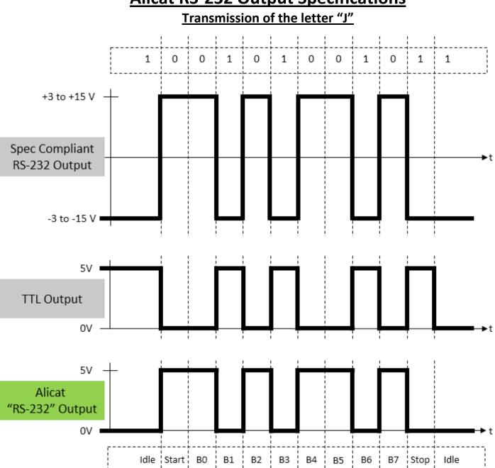
The Alicat RS-232 output uses the same timing as RS-232, and outputs a high voltage that is within the +3V to +15V range for RS-232, but outputs an idle and low voltage at 0V.
